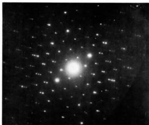
Fig. 12. Focused point diffraction pattern with the incident beam at a high inclination to the c axis, so that the projected c spacing and projected \beta angle can be measured to identify the polytype as 2M .
